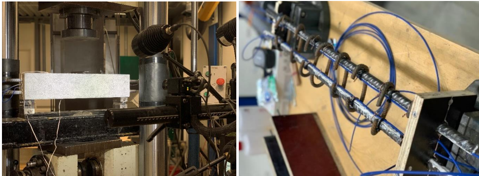
Figure 2. DIC system setup, with speckle pattern on the beam's front side (left), FOS in the rebars before casting (right).
